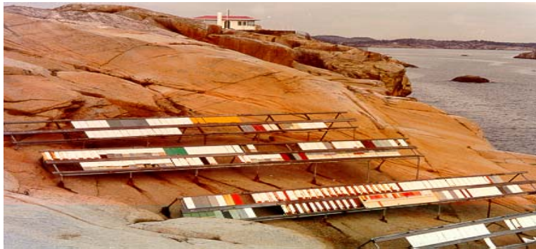
Picture 1. Marine paint test site south Norway.
