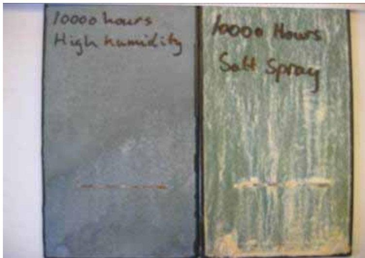
Picture 1. Ethyl silicate exposed for high humidity and salt spray for 10000 hours. The scribes are soon "repaired" and closed by zinc salt.
