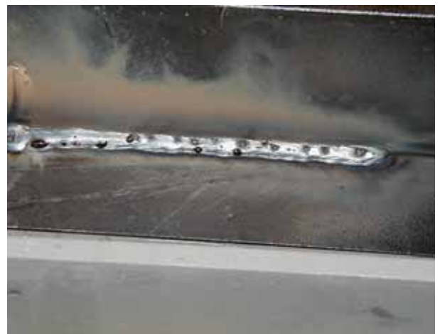
Picture 3. Seem after welding in inorganic shopprimer to the left and organic shopprimer to the right. The organic material forms gasses that create pores in the welding seem.
